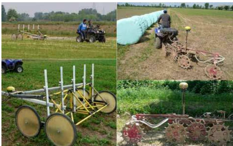
Figure 3.4: Geophysical instruments used during the survey. *Left* – the Automatic Magnetic Profiler (AMP © Geocarta), capable of recording up to 20ha/day. *Right* – the Automatic Resistivity Profiler (ARP © Geocarta), capable of recording up to 4ha/day. To increase productivity within the project two ARP instruments were often used simultaneously.
